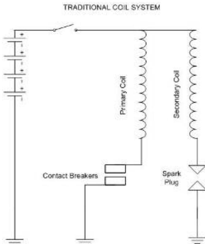
Since the advent of engine management, ignition coils have undergone a complete redesign. Gone are the traditional oil/asphalt filled, barrel shaped coils, now virtually all manufacturers use resin filled plastic coils which are manufactured in all shapes and sizes. They are smaller, lighter and more efficient but regrettably they are not always more reliable.
