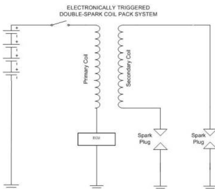
The traditional ignition reached its zenith. It became saturated at the higher voltages demanded from them and alternatives were sought. The higher voltages required to trigger the spark also caused
