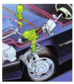
Citroen's hydractive suspension was first introduced on the XM and is a refinement of Citroen's justly famous oleopneumatic suspension first seen on the Traction Avant as long ago as 1952. It uses a central ECU to control the firmness of the suspension, cutting down roll and sharpening the reactions to the steering, while keeping the ride quality good.
