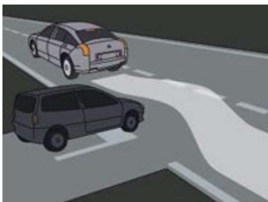
The Anti-lock Braking System (ABS) electronically regulates braking pressure to avoid wheel-locking so the driver can maintain road holding and the ability to steer the vehicle when braking.
