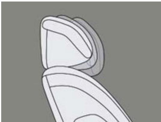
In the event of rear impact, the active front head restraints mechanism of the Citroën C6 reduces the risk of neck injuries. It works by automatically moving the headrest forwards towards the nape of the occupant's neck at the same moment as they are restrained by the seatbelt.
