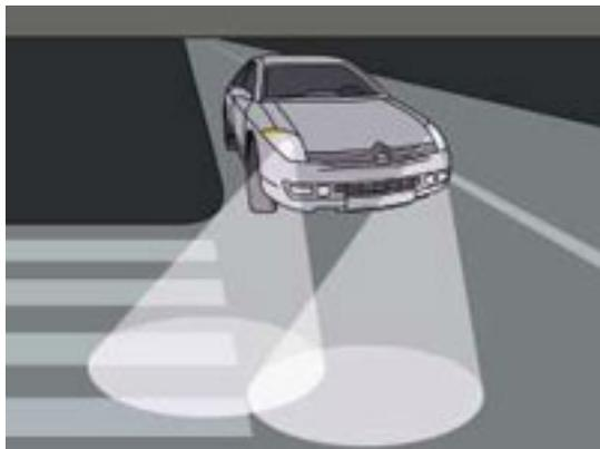
The Xenon dual function headlamps on the Citroën C6 use discharge lamp technology for dipped and full beam. The efficiency of the light intensity generated is further increased by the directional headlamps.
