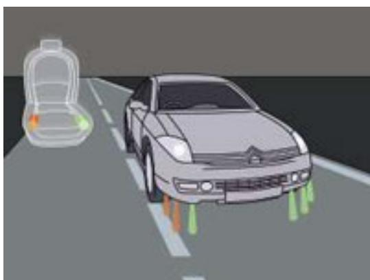
To prevent risks caused by any lapses in the driver's attention, the Lane Departure Warning System (LDWS) reacts to any inadvertent lane departure on a fast road.
