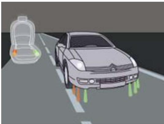
To prevent risks caused by any lapses in the driver's attention, the Lane Departure Warning System (LDWS) reacts to any inadvertent lane departure on a fast road.
