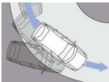
The ESP (Electronic Stability Program) operates automatically on the distribution of braking power together with engine speed to stabilise the trajectory of the car on bends as soon as any risk of oversteer or
