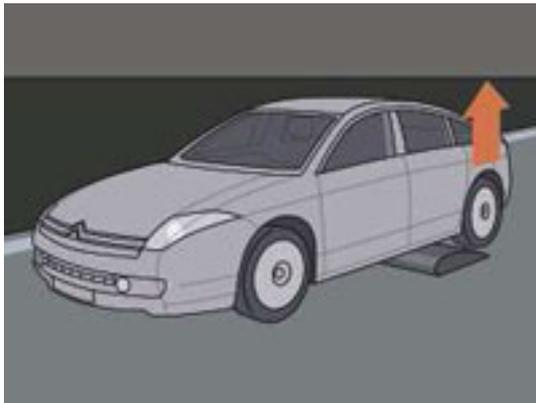
The efficiency of the Citroën C6's active suspension is reinforced by a variable damping system. Each wheel is fitted with a vertical wheel clearance sensor and an electronically adjusted variable absorber.
